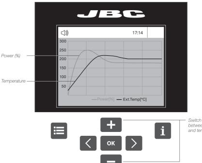
Switch Y axis between power and temperature
