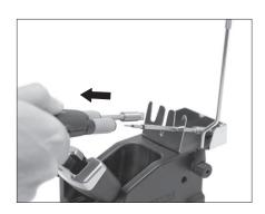
**4.** Follow the "Placing cartridges" guidelines. You can also use the extractor to insert the cartridges.
