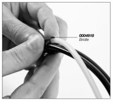
4 Strap the silicone tube to the handle cable and freeding tube, using the bridles, to make it more manageable.
