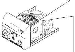
2. Install the valve and valve guard.
