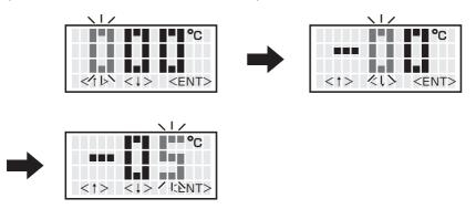
3. After entering the units digit, press the button to save the figure to the system memory and begin heater control with the new offset value.
