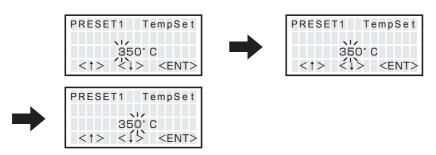
3. After entering the units digit, press the button to save the figure to the system memory and begin heater control with new setting temperature.
