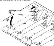
Measure the resistance of the heater. If the heater has an open circuit, replace the heater.
