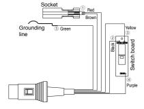
Checking the connection cord for breakage
