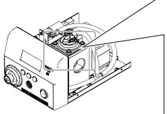
2. Install the valve and valve guard.
