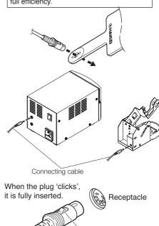
Push the plug in as far as it will go, and try to remove it without pressing the release pin. If it stays in the receptacle it is properly seated.
