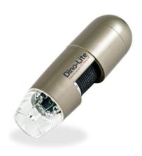
The AM4113T-FVW is suitable for inspection of paintings, ancient relics or other objects of art where UV light is required. It offers a high magnification (up to 200 times) and switchable LED lights – they can be switched from UV to white light. The UV light supplies an excitation of ~400 nm. It has a filter which blocks the returning UV light, resulting in images with natural colors.
