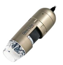
The AM4113TL-FVW is an ideal solution for inspection and working on objects of art where the usage of UV light is required. The long working distance of up to 15 cm enables the user to work under the microscope. This model offers a magnification of up to 90 times and switchable LED lights. The lights can be switched from UV to white light. The UV light supplies an excitation of 390~400 nm. It is equipped with a filter which blocks the returning UV light, resulting in images with natural colors.
